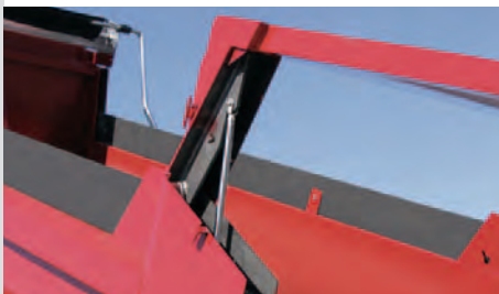
Power tailgate creates an opening 18" higher than tailgate itself.
