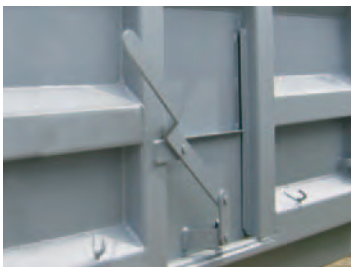
Traditional sliding rear patchgate features easy operation.
