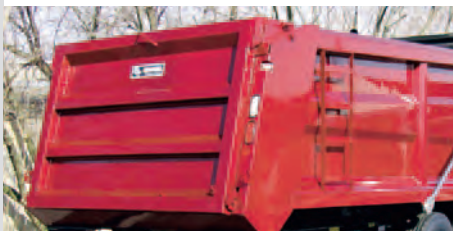
Asphalt tailgate eliminates the need for a spreader apron and allows you to pull away from the paving unit while the body is raised.
