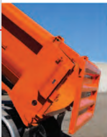
Performs like a standard tailgate and a high-lift tailgate, will also slide in tracks to allow metering of asphalt and spreading of gravel.
