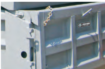
Straight rear with horizontal and vertical tailgate braces.
