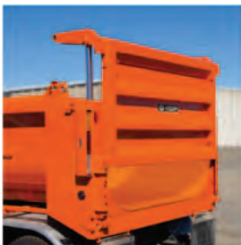
Performs like a standard tailgate and a high-lift tailgate, will also slide in tracks to allow metering of asphalt and spreading of gravel.
