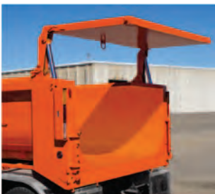
Performs like a standard tailgate and a high-lift tailgate, will also slide in tracks to allow metering of asphalt and spreading of gravel.
